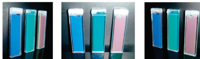
FIGURE 2. Optical images of gel particle suspensions with different polymer contents. These images were taken at angles different from the direction of incident light.
